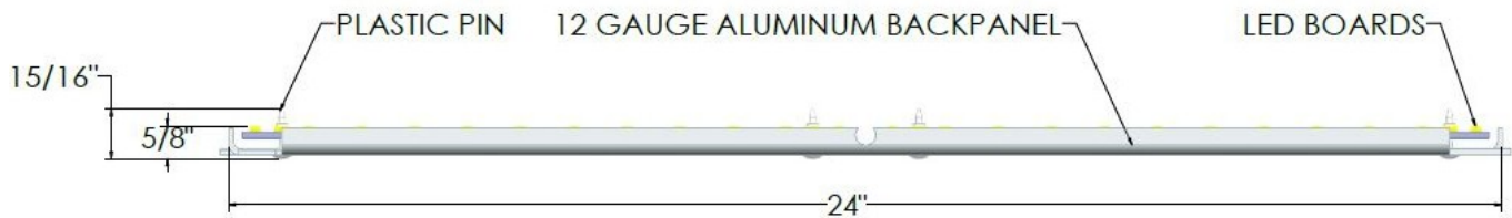
Fig 5: Typical aluminum back panel cross-sectional detail
