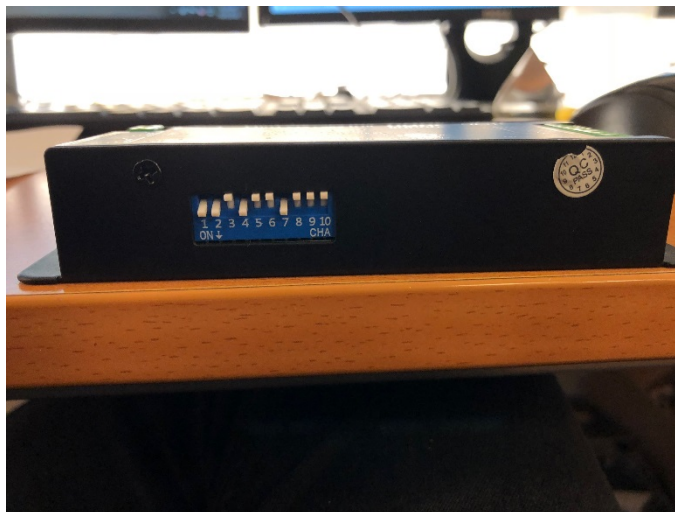
Image 6 : 1,2,4 & 7 number DIP Switch position TURNED ON for DMX address 75 onto DM4 Module
